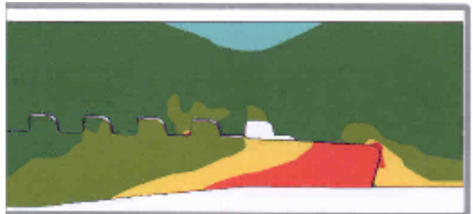
Fully Made-up with Pin Shouldering & Preloaded
