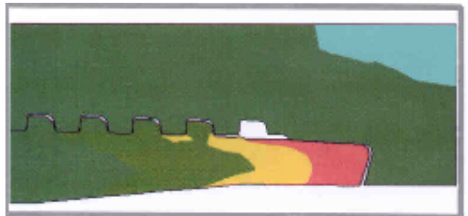
Second Stage Seal & Thread Interference up to shoulder
